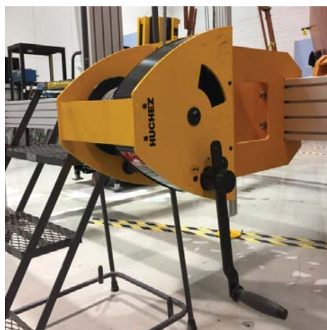
FIG. 4. Huchez Manibox GR1000 winch provided to rotate RICH.
