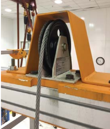
FIG. 5. Gebuwin KB1000 pulley provided for RICH rotation. The pulley has a maximum load capacity of 1000 kg. Maximum wire rope diameter allowed is 10 mm.
